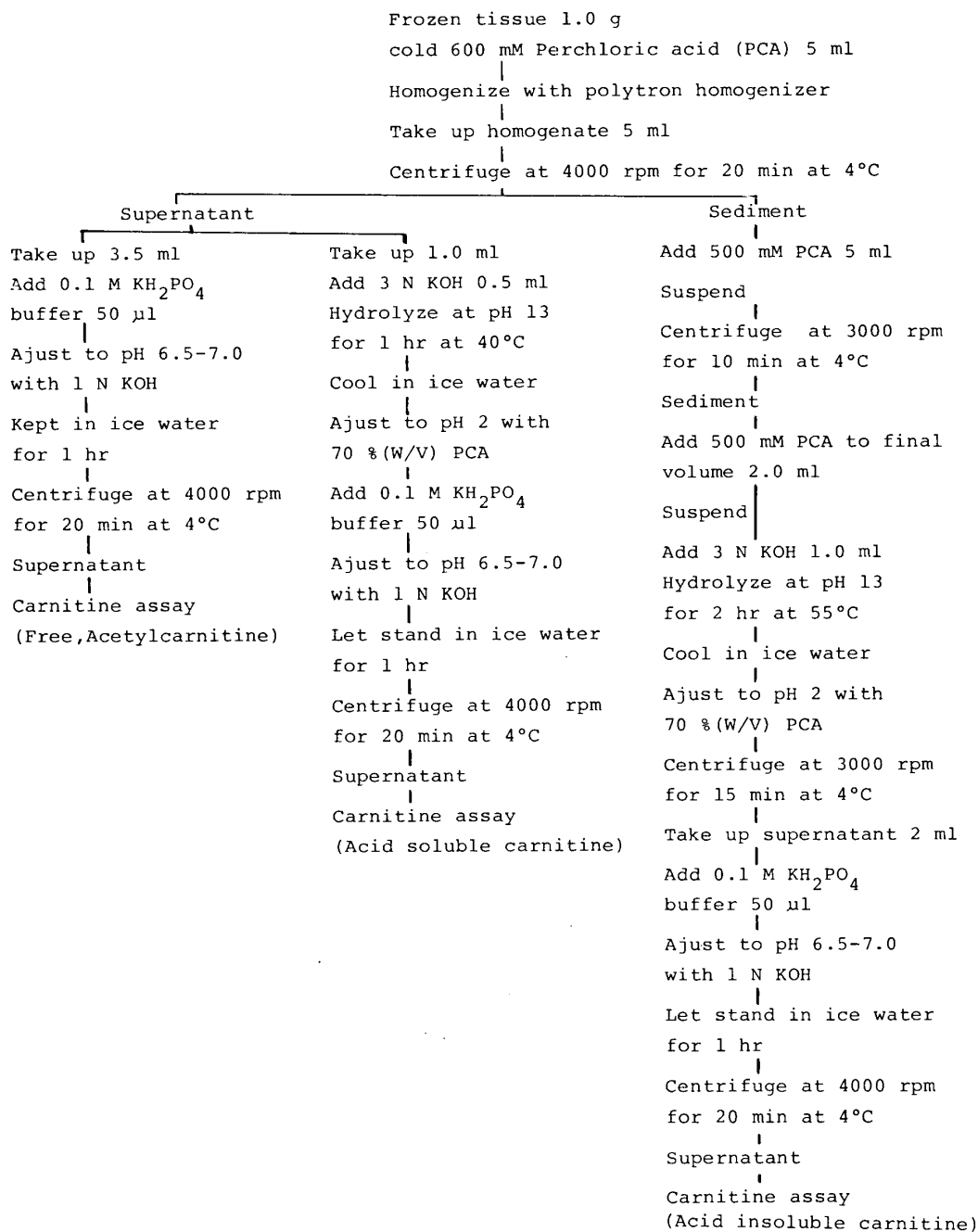
Fig.2. The extraction of carnitine and its acyl derivatives. Acid soluble carnitine = free carnitine + short chain acyl carnitine; acid insoluble carnitine = long chain acyl carnitine; Short chain acyl carnitine includes acetylcarnitine. Total carnitine = acid soluble carnitine + acid insoluble carnitine.
