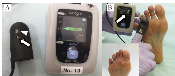
Fig. 1 Measurement of the regional hemoglobin oxygen saturation (rSO 2 ) using a finger-mounted tissue oximeter. (A) A finger-mounted tissue oximeter using the near-infrared spectroscopy technique (white arrow: optical source; arrow head: optical detector). (B) rSO 2 measurement at the dorsal side of the fourth toe near the ulcer (white arrow: rSO 2 value).
